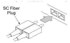
Figure 2-3. Inserting an SC fiber plug
